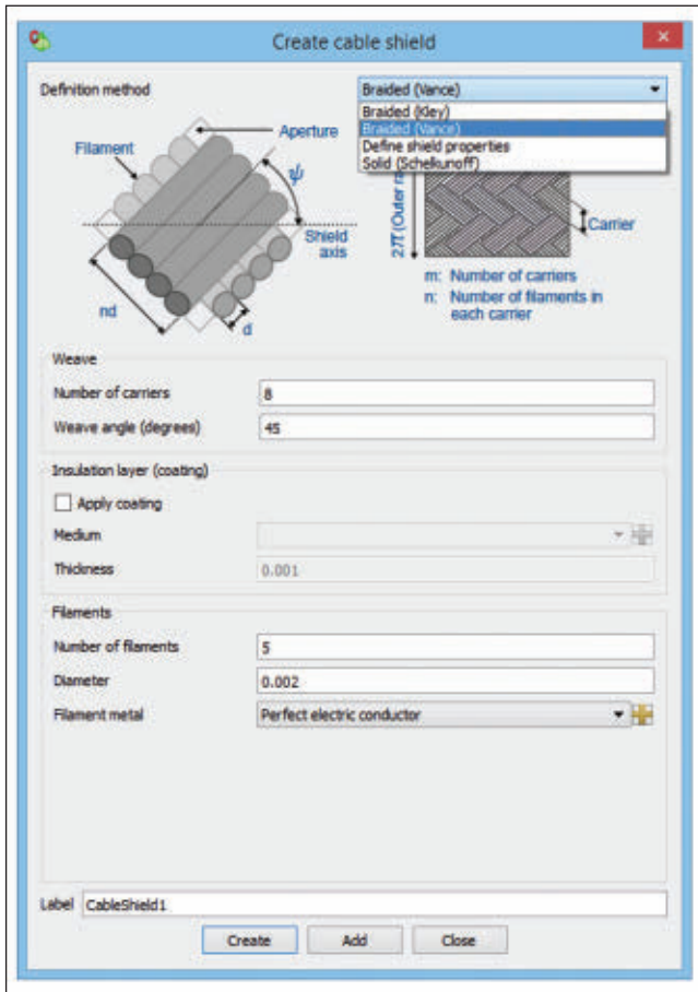
▲ Fig. 3 Create cable shield dialog in CADFEKO including the Vance braided shield type, added via the dropdown menu.
